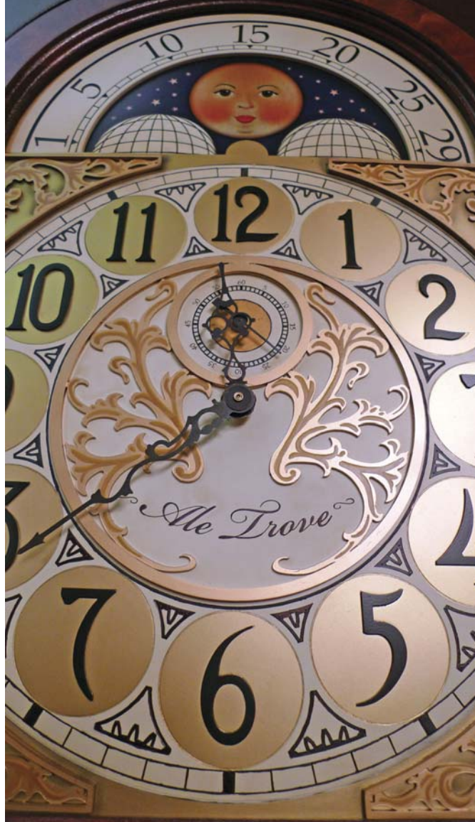
Above: A part of the Time Keeper's lair, this rafters set is an example of the interactive pieces that were designed to move quickly in and out of the small green stage by fork lift. Left: A detail of the grandfather clock face in the Watch Shop as the clock parts come together. Acrylic layers were cut on the Epilog Laser. Below it is the plan drawn by Set Designer Jeff Adams.
