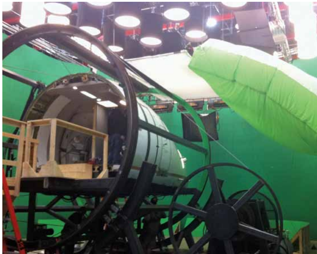
Above: The "rotisserie rig" designed to flip plane sections, here with the cockpit section installed, on stage in Atlanta.
