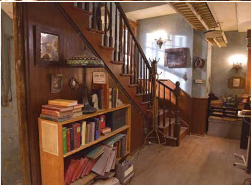
Three views of the interior stage set. Top: The completed and dressed pawn shop with actual pressed tin tiles for the ceiling. All counter and shelving units were put on wheels, and the bookcases rolled away with the wall units to open the set. Above, left: Another shot of the set from behind the loans desk, custom-built out of oak. Right: The rear stairs behind the loans desk leads to Setrakian's apartment. A lot of found doors and windows were used on this set which heightened its period feel and authenticity.
