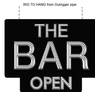
FRONT ELEVATION Double faced Neon Can Sign Scale: 1" = 1'-0" Paint lightly weathered charcoal/black Painted letters White Interior of profile extrusions - White
