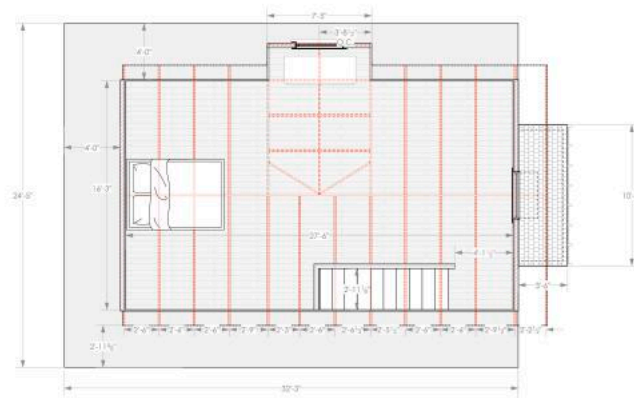
PLAN - PENNY'S ROOM - WITH BACKING SCALE 1/4" = 1'-0"
