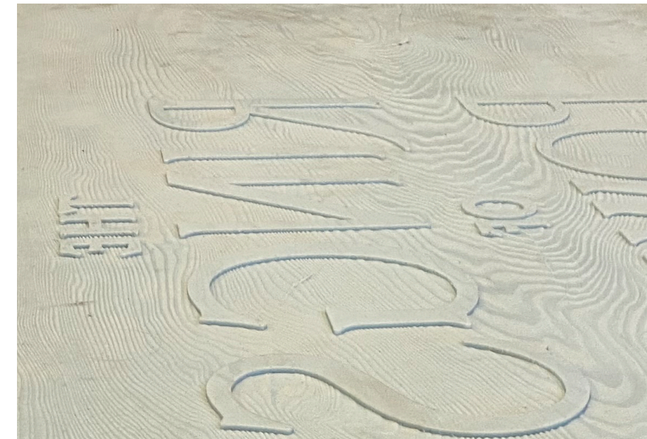
Silicone mold, retaining grain of wood
