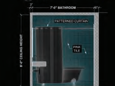
E-2 SECTION - BATHROOM 2.02 SCALE: 1/2" = 1'-0"
