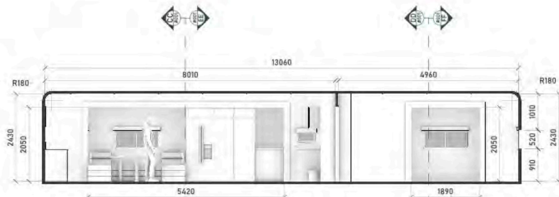
AA - LONG SECTION THRU TRAILER @ 'AA' SCALE: 1:50
