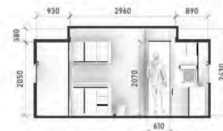
EE - CROSS SECTION THRU TRAILER @ 'EE' SCALE: 1:50
