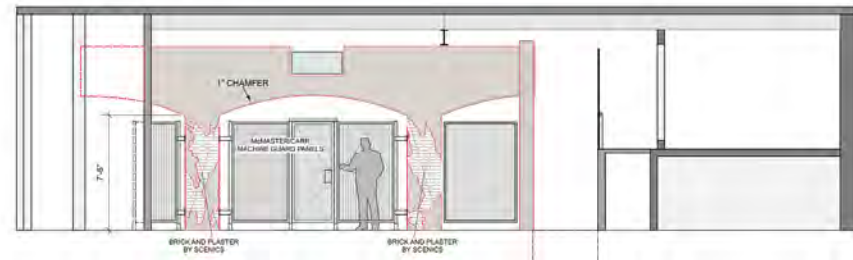
6 ELEVATION: OPEN ARCH - BACK SIDE Scale: 1/4" = 1'-0"
